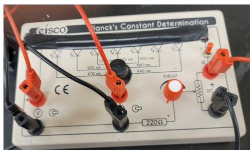
Fig. 1. Planck’s apparatus. On the left, leads go to a voltmeter. Center leads to an ammeter. Right leads to a power supply set at 9.00Volts. Either the potentiometer on the setup or fine voltage adjust on the power supply can be used to set the voltage applied to the LED.
